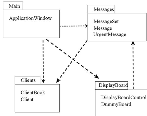
This diagram shows the four packages used and the classes within each package. Also shown are associations between the packages. Not surprisingly the main package, which houses the system interface, is associated with all of the other packages – this is because the interface invokes functionality throughout the system.
